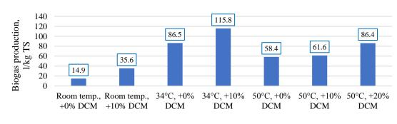
Figure 7. Biogas production
