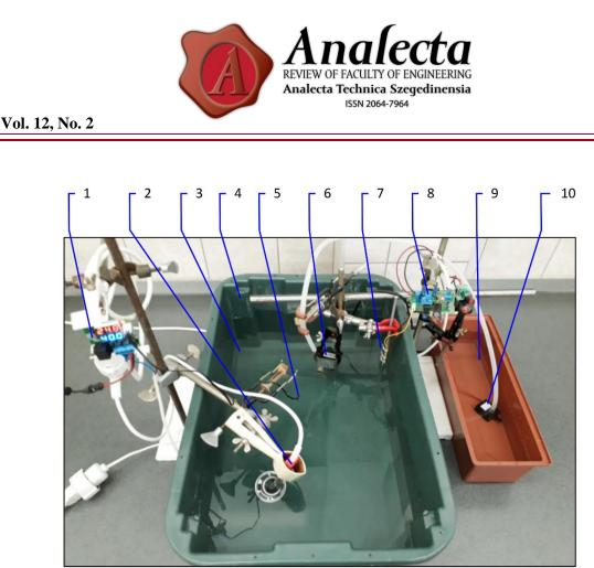
Figure 1. The temperature-regulated water bath system (1 – W1209 digital thermostat; 2 – immersion heater; 3 – water bath; 4 – PP harvest crate; 5 – NTC waterproof temperature sensor; 6 – aquarium pump; 7 – liquid level sensor; 8 – liquid level controller; 9 – replenisher for the water bath; 10 – submersible water pump)
