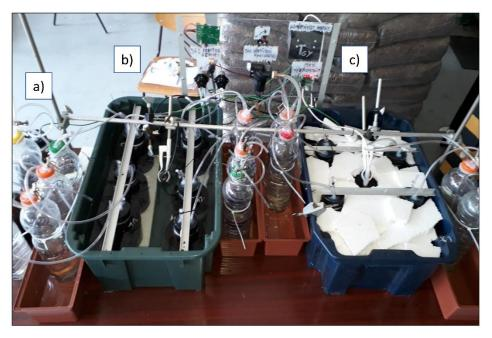
Figure 4. The assembled fermenter system with 2 reactors operating at room temperature (a), 6 at 34  $^\circ$ C (b) and 4 at 50  $^\circ$ C
