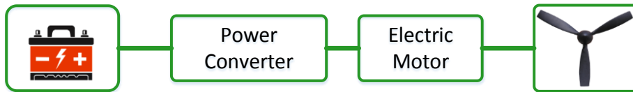
Figure 2. Block diagram of all electric propulsion system
