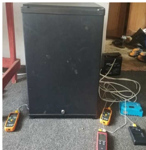
Figure 5. Vapour Absorption Cooling System developed under testing period condition
