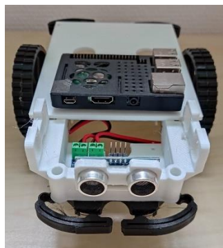
Figure 2. 3D printed and assembled mobile robot platform.
