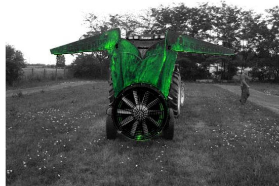
Photo 8. Contamination on the Sprayer (Modified Picture)
